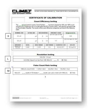
The test page is supplied with ISO 21501-4 compliant calibrations.
