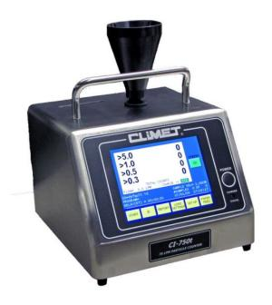
It has been called the *horn, the megaphone, the funnel,* and even *the big sucky thing.* Occasionally it is called a sample probe. Officially, it is an *isokinetic sample probe. Isokinetic* means that in a laminar flow area, the air flows in and around the probe without creating any turbulence.
