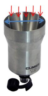
However, due to the inertia of 5  $\mu$ m and larger particles, there is significant loss of 5  $\mu$ m particles in the transport tubing. Some have tried sampling without a probe, but they are just exchanging loss of 5  $\mu$ m particles in the transport tubing for a loss of 5  $\mu$ m particles for lack of a wide enough opening to entrain the 5  $\mu$ m particles; only 5  $\mu$ m particles in a narrow cone above the inlet will enter the particle counter.
