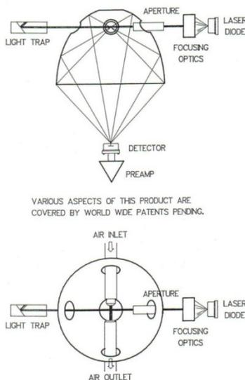
One of the many patents obtained by Climet is a metal ellipsoidal mirror used in our laser optics. This technical innovation provides us a superior competitive advantage.
