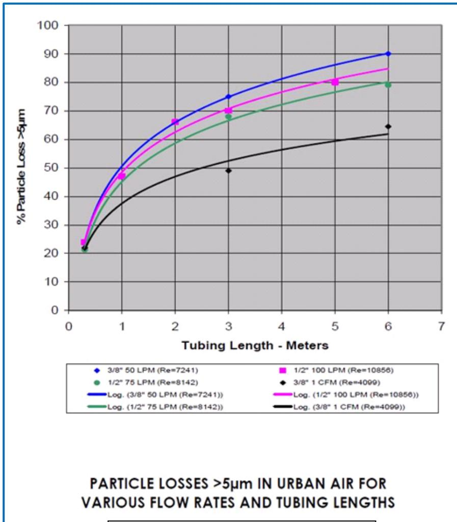
As a consequence of Climet validation procedures, Climet recommended a shorter transport tubing length for a 100 LPM particle counter of 2 meters (~6 feet) maximum.
