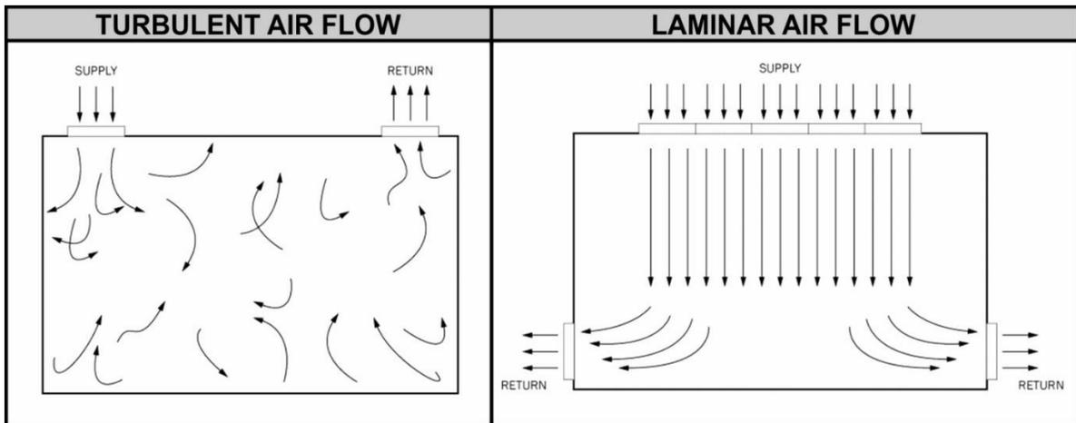
Isokinetic sampling is required in laminar flow (aka unidirectional flow) areas.
