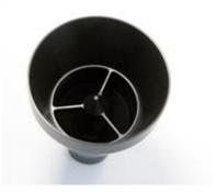
A unique, aerodynamic design avoids impaction losses; the light blocking element pulls particles around it, avoiding impaction.
