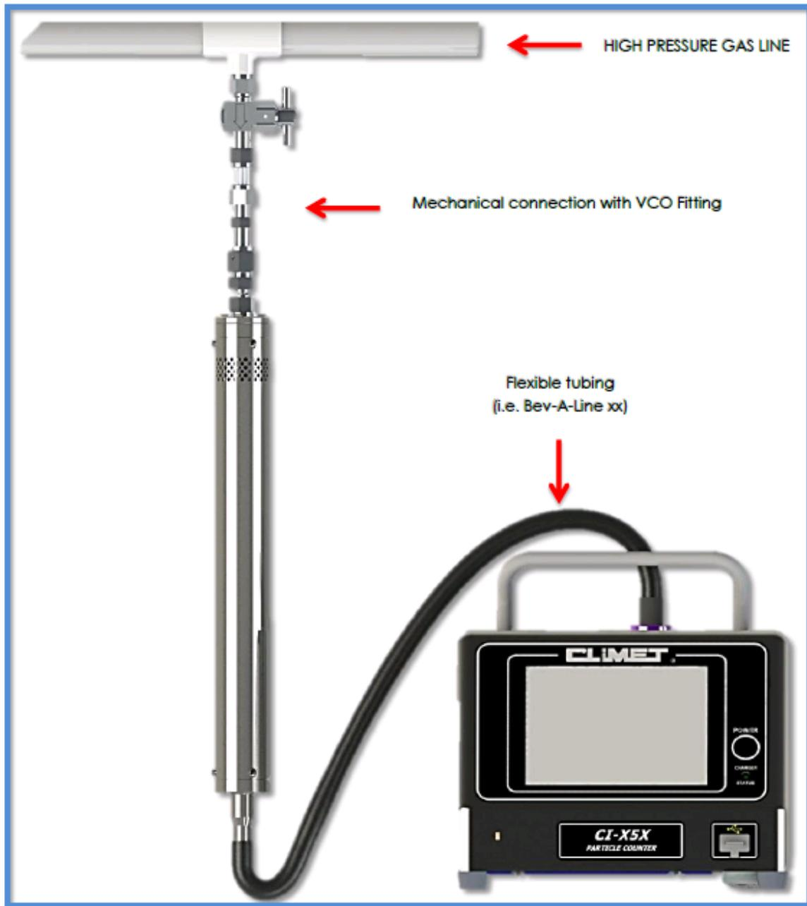
The location of the test point should be after the regulator and HEPA filter on the high pressure line. Tubing length should be 10 feet to mitigate high counts associated with sonic waves, and no sharp bends (Image above is for demonstration purposes only). Climet recommends use with a 1 CFM, 50 LPM, 75 LPM, or 100 LPM flow rate particle counter or microbial sampler.
